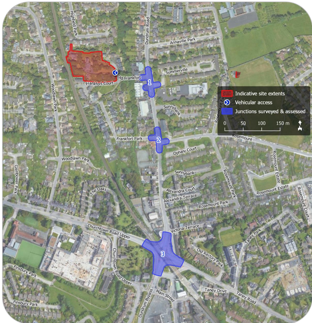
Figure 3 – Surveyed road junction sites (map data and imagery: OSM Contributors, Google)
